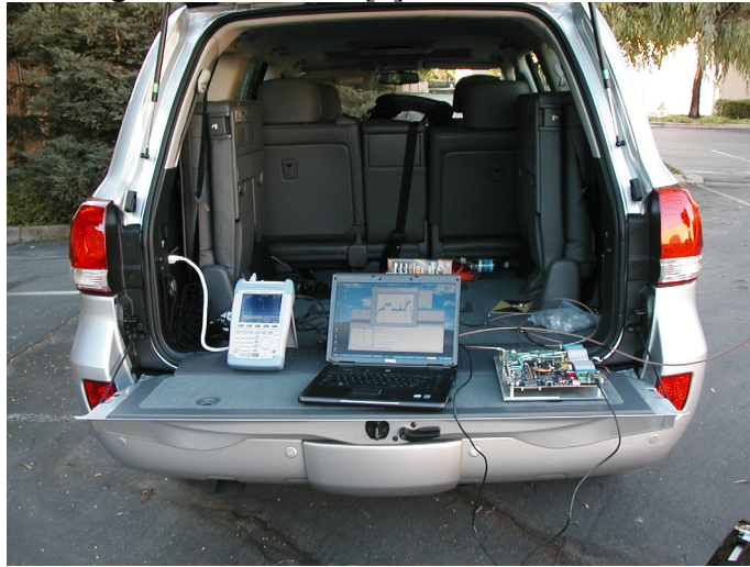
Figure 5: Wireless microphone beacon detection setup.
