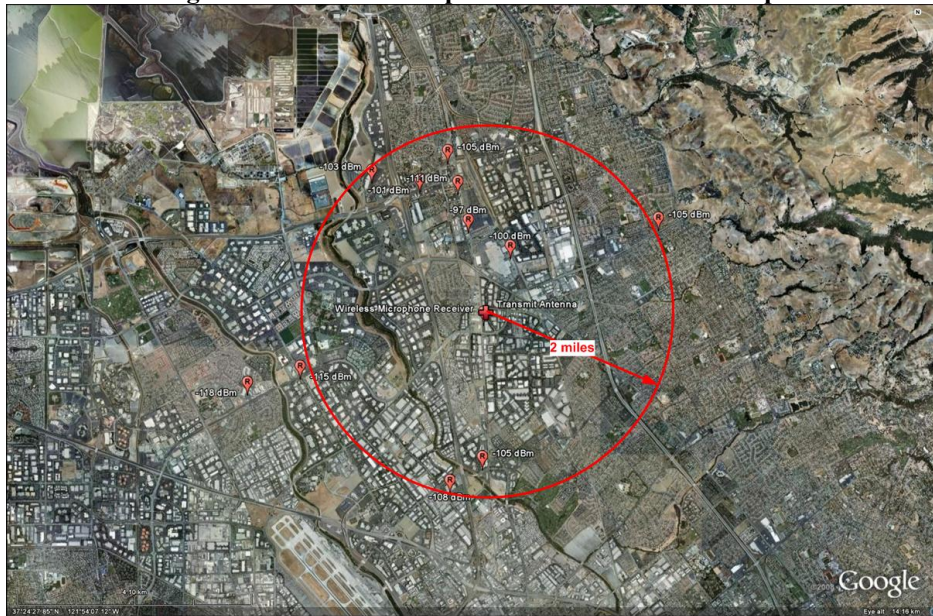
Figure 6: Beacon range measurement results.
